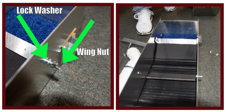
**Step 2: Attach Header Box to Sluice Box**
